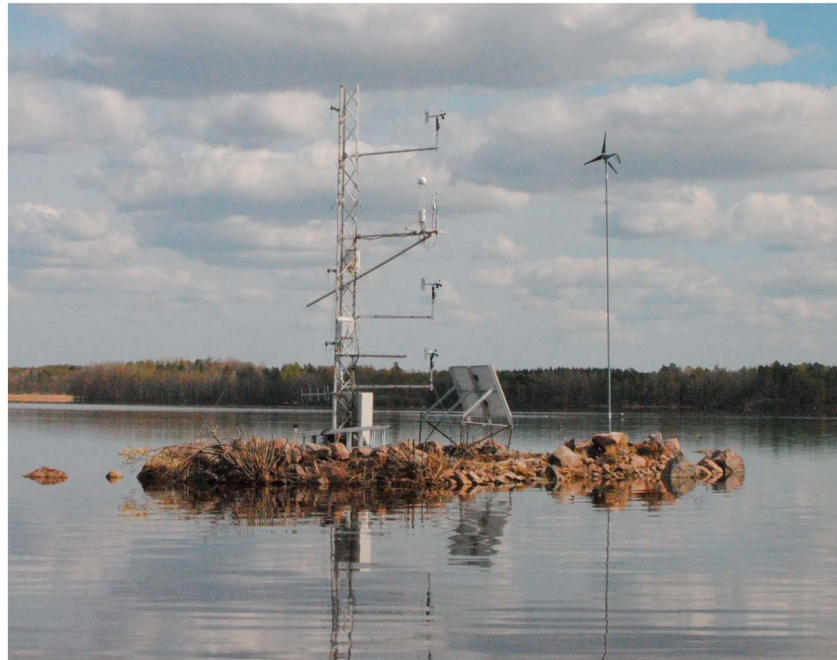
Figure 2. Rättarharet Island facing east, showing the 6 m tower with the instrumentation, solar panels, and wind turbine for the power supply.
